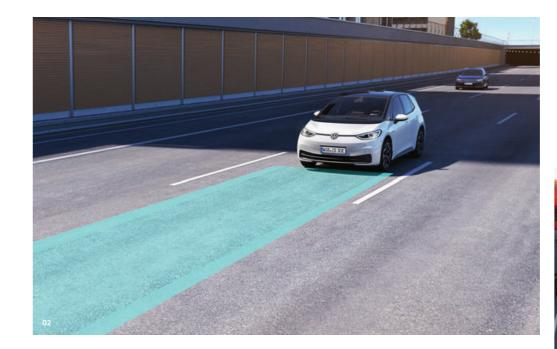
02 As from a speed of 60 km/h, the optional lane keeping system Side Assist can detect whether the ID.3 is unintentionally straying from its lane. In this case, it can direct the driver's attention back to the road with a corrective steering intervention.<sup>2</sup>
