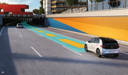
03 At the touch of a button, Travel Assist ensures a high level of driving comfort by providing support in monotonous or tiring conditions: on motorways and major country roads in particular, Travel Assist can maintain the lane and speed, as well as the distance from traffic ahead. This allows you to stay relaxed when stuck in traffic jams and stop-and-go traffic.<sup>2</sup> SO
