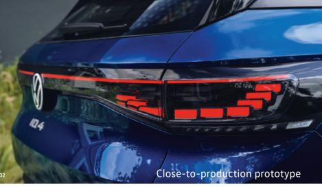
**02** A thin strip of light extends above the characteristic 3D LED tail light cluster with dynamic turn signals all the way to the new Volkswagen logo.
