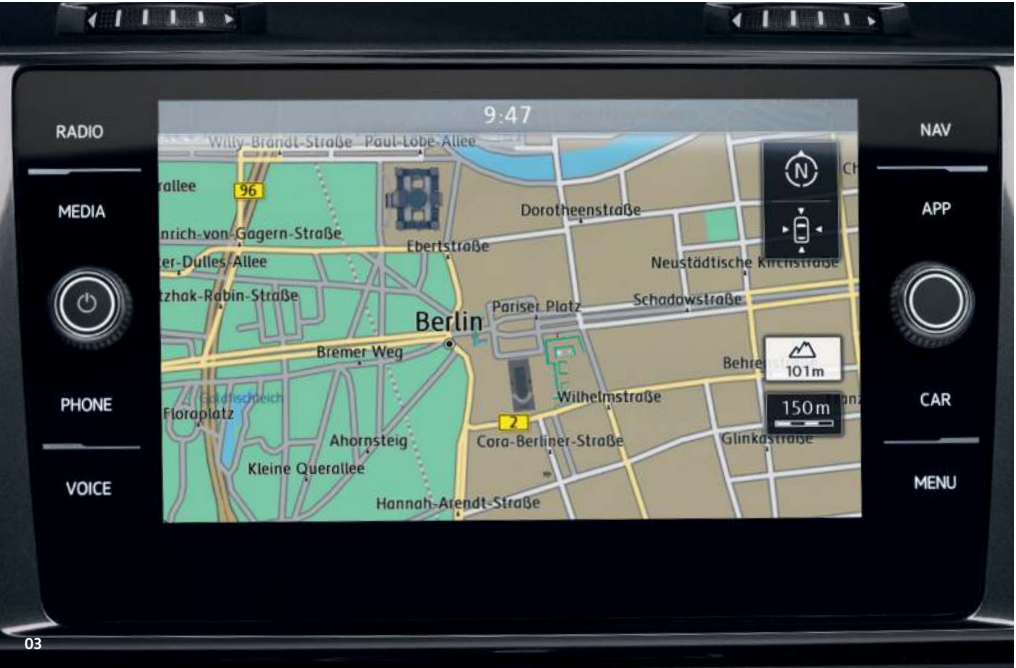
04 Discover Pro navigation radio system. The 'Discover Pro' touchscreen navigation radio system features a glass-covered 9.2 inch colour touchscreen for navigation and radio functions. It responds to spoken voice commands for navigation and telephone functions. Building on the 'Composition Media' specification, it is equipped with a 30 GB SSD hard drive, preloaded European navigation data, 3D map view, three calculated routes (Fast, Short and Eco), points of interest, Speed Limit Display 2 , photo display from JPEG and PNG files and two SD card readers. It comes with 3-years We Connect 'Guide and Inform Plus' 3 , providing online access to such information as fuel pricing, parking space availability, weather and news feeds; and includes online navigation software updates, enabling you to download the latest map data. Optional on Highline and R-Line models.
