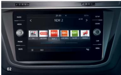
02 Composition Media radio system. The 'Composition Media' system is equipped with an impressive glass covered 8.0 inch colour touchscreen with a proximity sensor that recognises in advance your intention to touch the screen and automatically magnifies the display mode. Features also include USB connection for compatible products and SD card reader. The media system also includes Bluetooth telephone and audio connection for compatible devices 1 , simultaneous pairing of two compatible mobile devices, SMS functionality – allowing you to read, compose and send SMS messages using the touchscreen display to a compatible Android smartphone (while the vehicle is stationary), title and compatible cover art display and facilitates music playback from MP3, WMA and AAC files through eight speakers, front and rear. Standard on Comfortline and optional on Trendline models.
