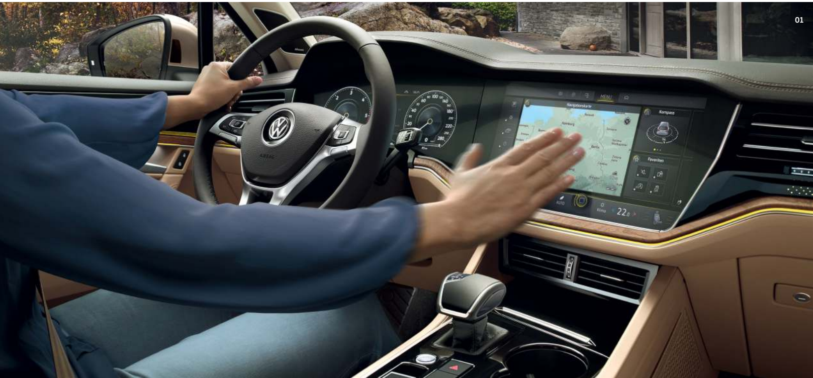
01 Gesture Control. With the optional innovative gesture control function, you have a simple and convenient way to operate the 'Discover Premium' or 'Discover Pro' navigation system. You can control a number of menu options with a simple horizontal gesture. For instance, you can switch to the next song or radio station by just waving your hand.
