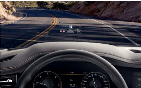
04 'The Head-up Display'. The 'Head-up Display' can show vehicle information directly in the driver's line of sight. The speed, road signs, driver assist system functions, warnings and navigation instructions are projected onto the windshield. This lets you read all the important information immediately while retaining your focus on the road. Available on all models.
