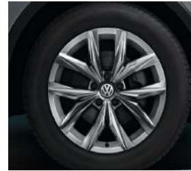
STANDARD ON HIGHLINE 18" Kingston alloys 7.5Jx 18 alloy wheels. Tyres 235/55 R18 low rolling resistance tyres
