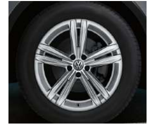
STANDARD ON R-LINE 19" Sebring alloy wheels 8.5J x 19 alloy wheels. Tyres 255/45 R19 low rolling resistance tyres
