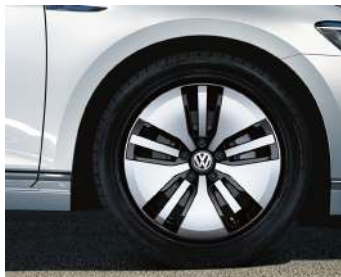
STANDARD ON GTE 17" 'Montpellier' alloy wheels 7J x 17 Tyres: 215/55 R17
