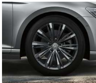
OPTIONAL ON R-LINE & GTE 18" 'Liverpool' alloy wheels in Admantium Dark 8J x 18 Tyres: 235/45 R18
