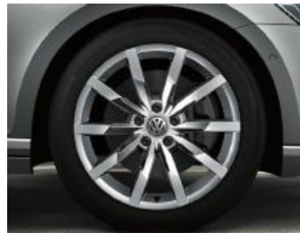
STANDARD ON R-LINE 18" 'Monterrey' alloy wheels in grey metallic 8J x 18 Tyres: 235/55 R18
