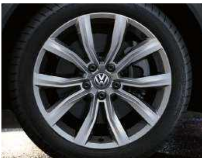
OPTIONAL ON SPORT & R-LINE 18" Moonboot alloy wheels with low rolling resistance tyres 7J X 18 Tyres: 215/50 R18
