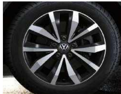
OPTIONAL ON DESIGN 17" Rebell alloy wheels in Black with low rolling resistance tyres 7J X 17 Tyres: 215/55 R17
