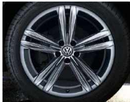
OPTIONAL ON R-LINE 18" Sebring alloy wheels with low rolling resistance tyres 7J X 18 Tyres: 215/50 R18
