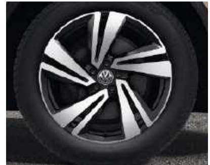
OPTIONAL ON TOUAREG & ELEGANCE 20" 'Nevada' alloy wheels, in 'Black' with diamond turned surface 9J x 20 Tyres: 285/45 R20 Note: Not available on Elegance PHEV
