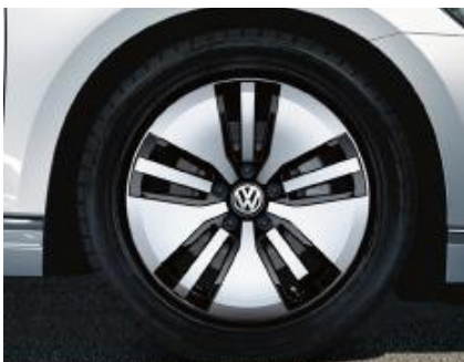
STANDARD ON GTE 17" 'Montpellier' alloy wheels 7J x 17 Tyres: 215/55 R17
