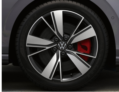
STANDARD ON GTD OPTIONAL ON GTE 18" 'Bakersfield' alloy wheels 7.5J x 18 Tyres: 225/40 R18
